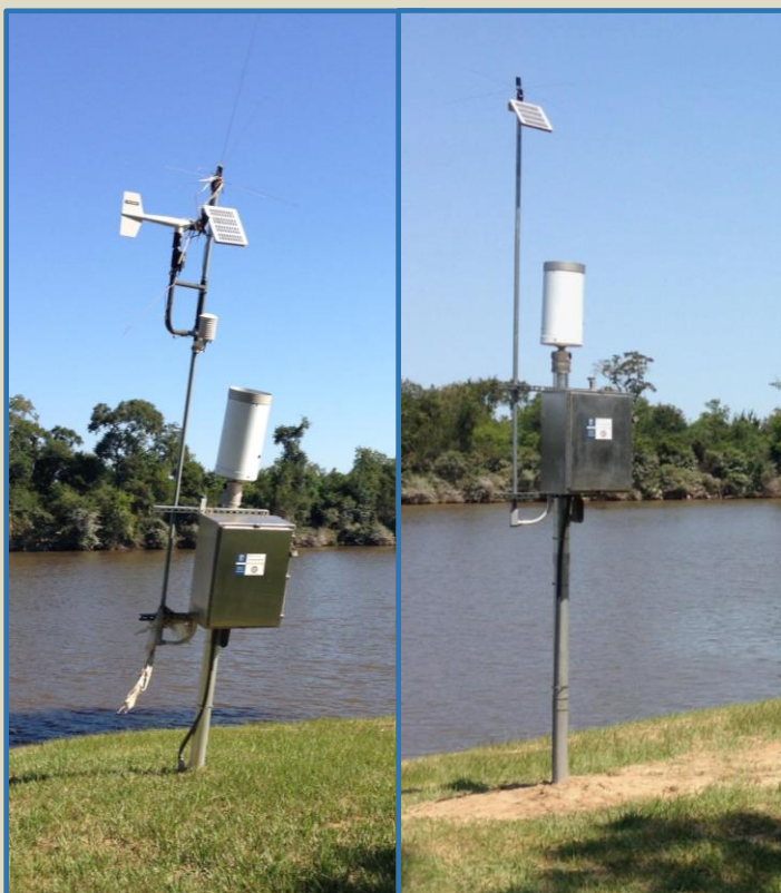
Figure 1. Flood gage along the banks of the San Jacinto River. Storm debris can be seen all the way to the top of the antenna mast. Repair work involved elevating equipment to prevent damage from future minor floods.
