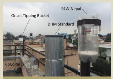
Figure 2 - Rainfall comparison between different gauging.
