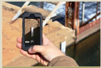
Figure 3 - Stage data collection with smartphone camera.
