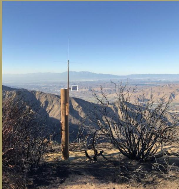
The Riverside County Horsethief Canyon ALERT2 Precipitation Station was recently installed to help provide advanced notice of conditions leading to post-fire debris flows and flooding.
